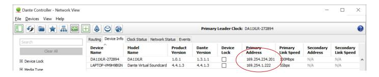
By accessing the IP address of the DA11XLR in your web browser, you will gain access the the units web GUI. The following details will allow you to log in to the admin section:
