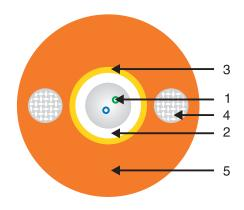
Twin G657a Fibres with PP outer sheath
